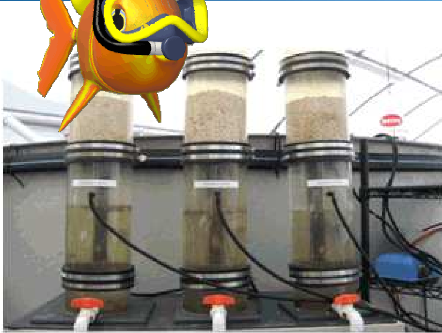
Figure 1. Three lab-scale PolyGeysers® denitrification units.
